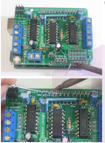
Solder in each pin of the header.
