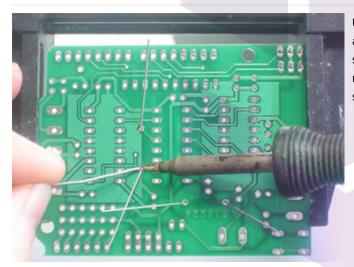
Using your soldering iron tip, heat the resistor wire lead and the metal ring (pad) at the same time, after a few seconds, poke a little solder in so that it melts into a nice cone. Remove the solder and then remove the soldering iron. Do this for all 4 wires.
