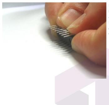
Next are the three integrated circuits (ICs) **IC1**, **IC2** and **IC3**. When ICs come from the factory, the legs are angled out somewhat which makes it difficult to insert them into the PCB. Prepare them for soldering by gently bending the legs against a flat tabletop so that they are perfectly straight.
