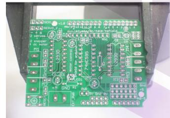
Place the motor shield PCB in a vise or other circuitboard holder and turn on your soldering iron to 700 degrees.
