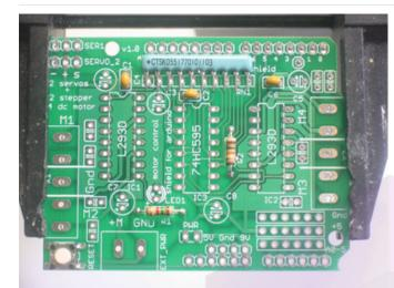
Next is the 6mm tactile switch**RESET** and the resistor network**RN1**. The tact switch is used to reset the Arduino since its not possible to reach the reset button once the motor shield is on.
