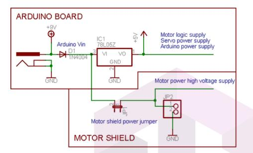
If you would like to have a **single DC power supply for the Arduino and motors**, simply plug it into the DC jack on the Arduino or the 2-pin PWR\_EXT block on the shield. Place the power jumper on the motor shield. If you have a Diecimila Arduino, set the Arduino power source jumper to EXT.
