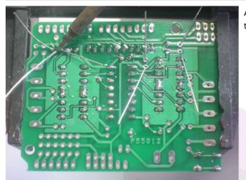
After double-checking their polarity, solder and clip the three capacitors.
