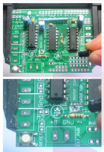
Place the two 47uF remaining electrolytic capacitors, **C7** and **C8**
