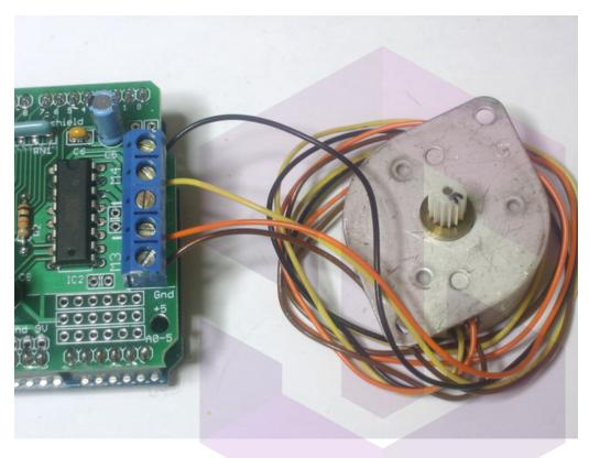
Stepper motors are great for (semi-)precise control, perfect for many robot and CNC projects. This motor shield supports up to 2 stepper motors. The library works identically for bi-polar and uni-polar motors
