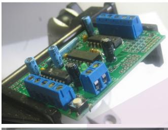
The 2 3-pin pieces go in the servo connections in the top left corner. The 2-pin piece goes in the PWR jumper in the bottom center.
