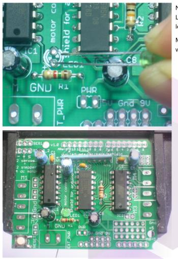
Next is the 3mm LED used to indicate motor power. LEDs are polarized, just like capacitors, and the long lead is the positive (+) lead.
